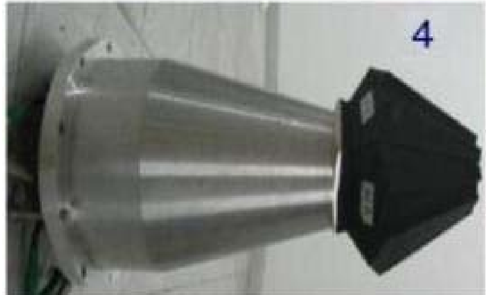
Elements of gamma multiplicity filter (BaF 2 ) ( not in use at the moment )
